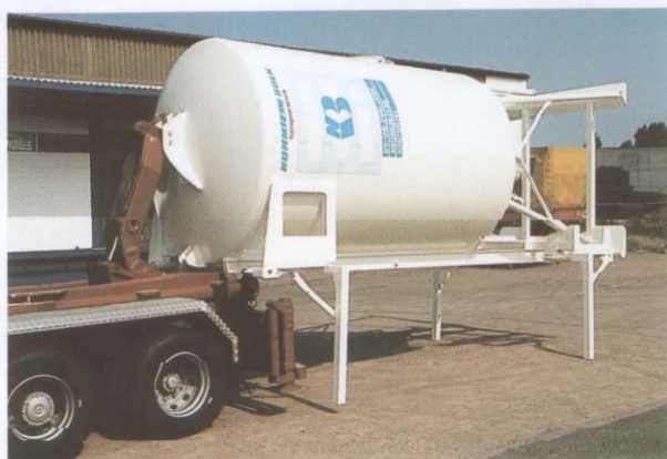
Mobile silo WS (ID) 22.5 for rail transport in accordance with UIC norms and road transport
