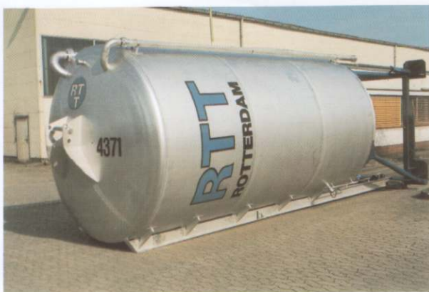
Special steel portable silo EWS (ID) 26 in free fall and pressure construction
